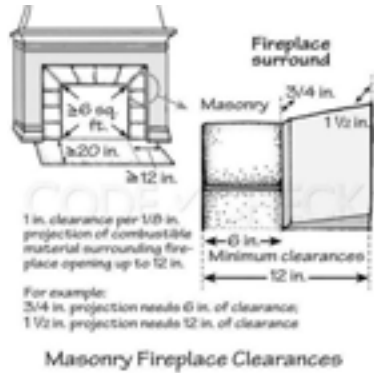
Masonry Fireplace Clearances
